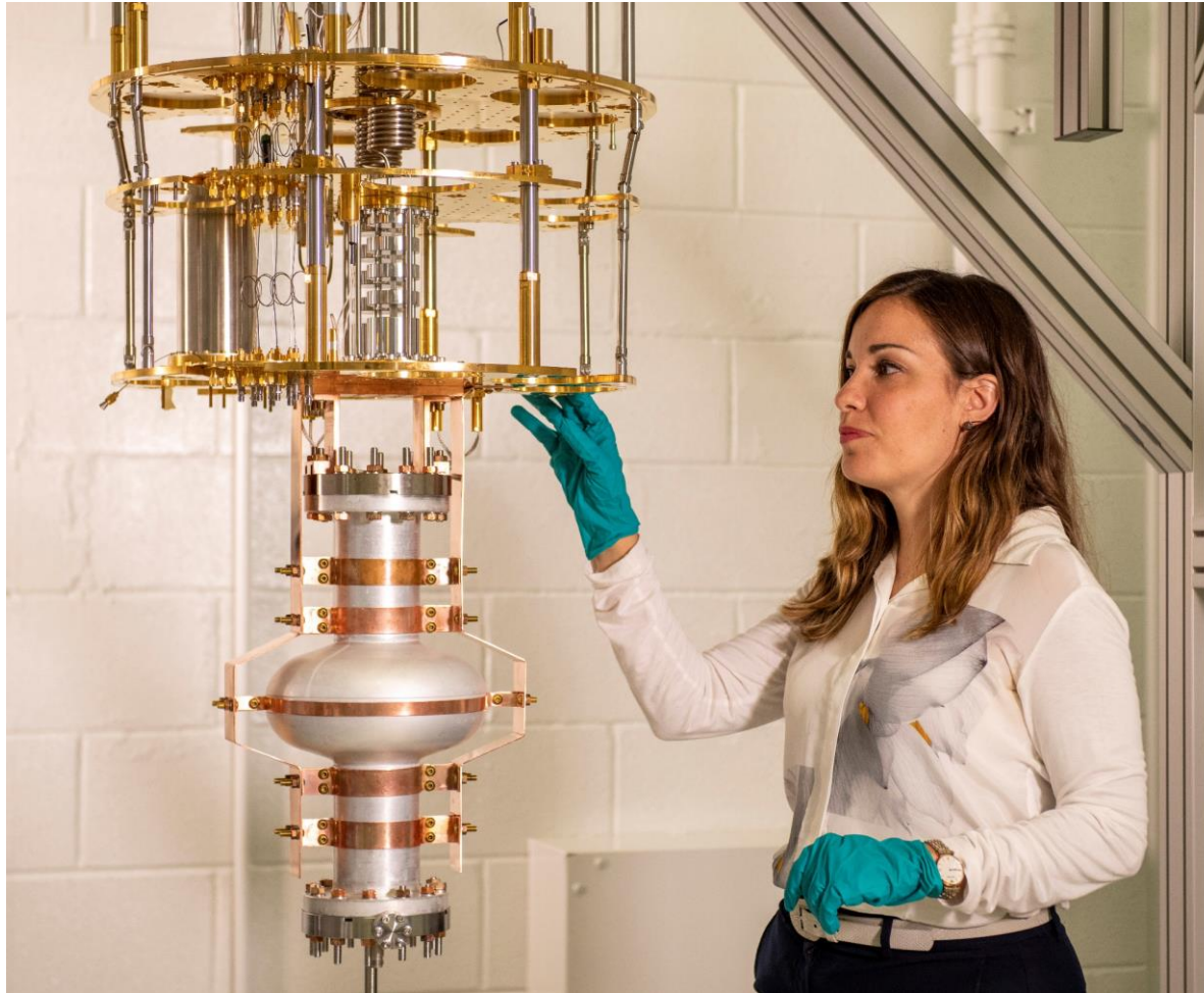
Dilution refrigerator set with an aluminum cavity in FermiLab
